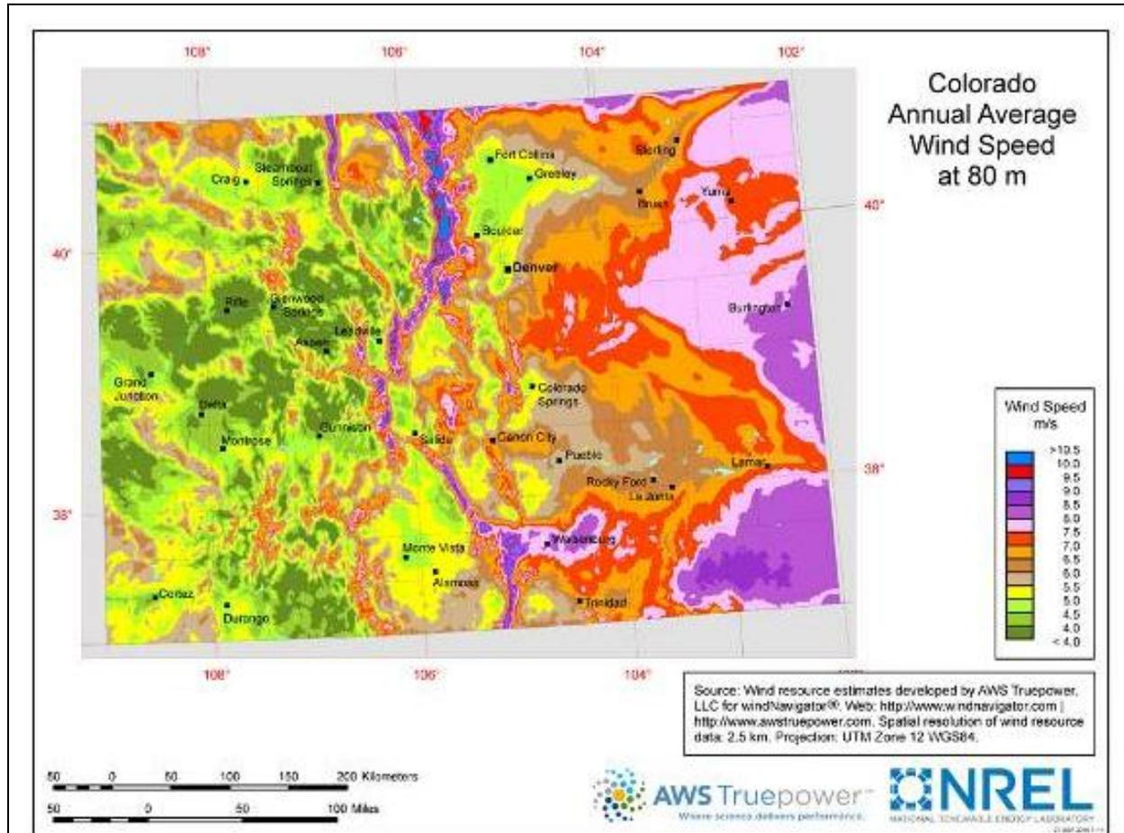
**Figure 8.1.** Colorado annual average wind speed (80m agl) suggests that the majority of wind development will occur on the Front Range and eastern plains (National Renewable Energy Laboratory, <https://windexchange.energy.gov/maps-data/15>, Accessed December 2017).
